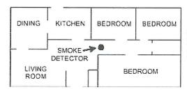
A smoke alarm should be located between the sleeping area and the rest of the family living unit.
